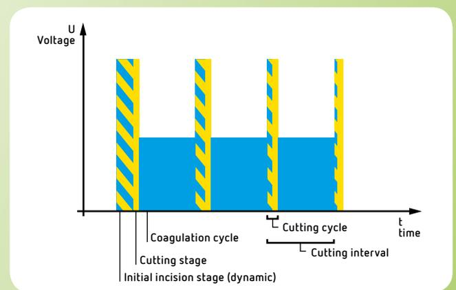
Cutting cycle with ENDO CUT® Q:
