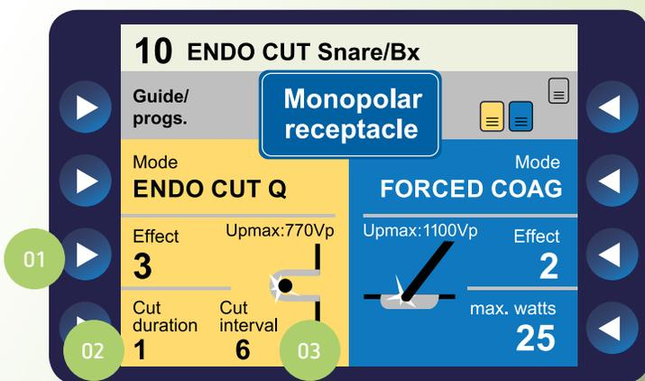
The coagulation phase allows for additional coagulation between the cutting phases. Coagulation intensity can be adjusted using the EFFECT setting, altering coagulation voltage levels. Raising the EFFECT setting increases coagulation intensity.
