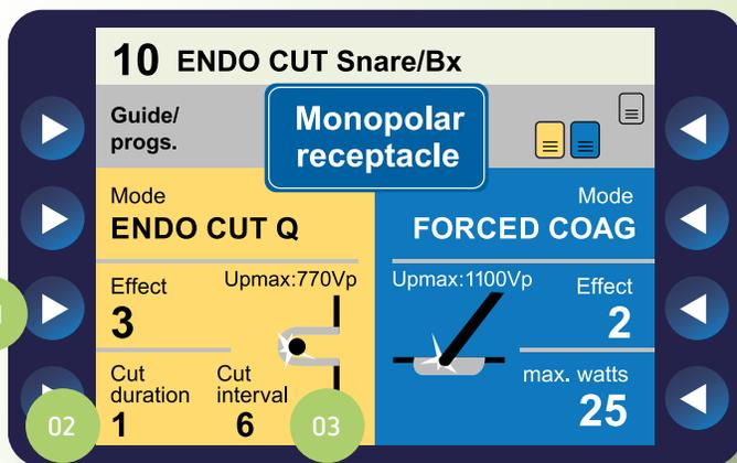
The coagulation phase allows for additional coagulation between the cutting phases. Coagulation intensity can be adjusted using the EFFECT setting, altering coagulation voltage levels. Raising the EFFECT setting increases coagulation intensity.
