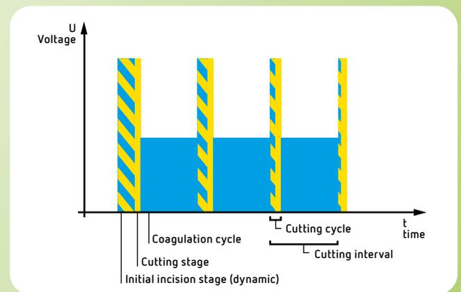
Cutting cycle with ENDO CUT<sup>®</sup> Q:
